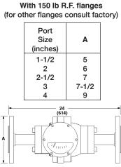
"Flow up" or "flow down" dimensions are the same. Scale numbers are turned 90° to be right reading. For additional information on flanged connection see page 129.
