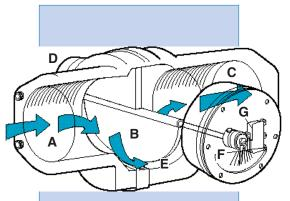
Fluid enters at A, passes around the semi-circular vane B. exits at outlet C. The vane resists the flow because of the spring D. The further the vane is pushed the larger the passageway E becomes. This minimizes pressure drop. The vane shaft turns to operate the pointer F and remote signal devices such as the switch G.
