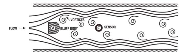
When fluid passes by a bluff, oscillations occur. Examples of these oscillations in nature include the swirls produced downstream of a rock in a rapidly flowing river, or the waving of a flag in the wind with the bluff being the flag pole.
