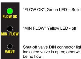
Shut-off valve DIN connector light is ON to indicated valve is open; otherwise, there will
