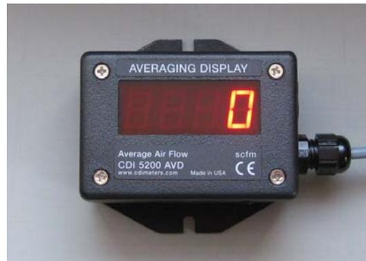
In most industrial applications, compressed-air flow changes constantly as loads turn on and off and as compressors load and unload. Usage is more accurately judged from a steady average than from a fluctuating rate display.
